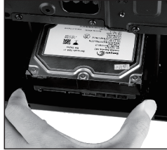
Put HDD bracket in the tool free,insert disk drive
