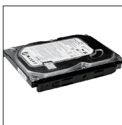
Fix HDD hard disk with free button (L/R)
