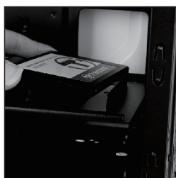
Put it on SSD and align the hole
