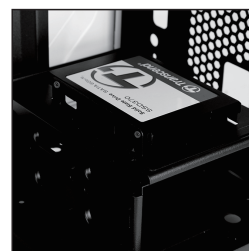
Screw the SSD from both sides
