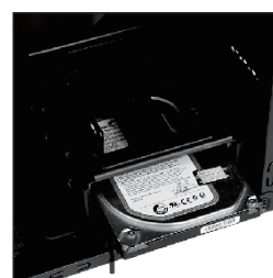
Align the hard disk with the hole and push
