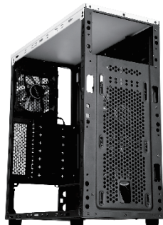
Fix Fans by fan Screws
