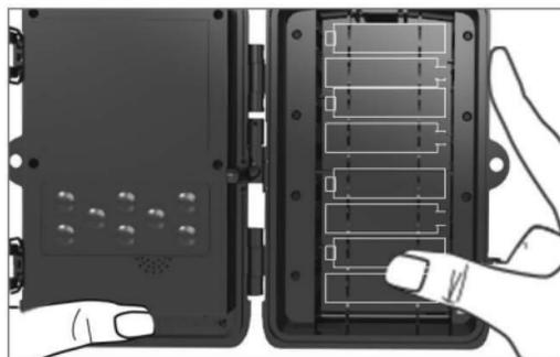
**NOTE:** Installing any of the 8-AA batteries in the wrong direction may cause the batteries to leak acid and could possibly explode, causing camera failure and damage to the battery compartment.
