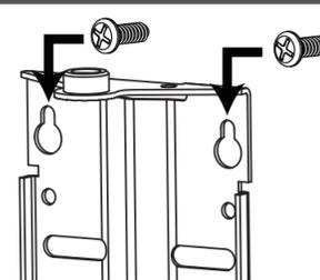
Drill holes and fix screws in the wall according to the holes position on the antenna bracket, attach bracket to the wall and secure with screws.
