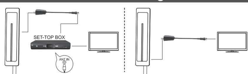
Connect the signal cable from the antenna to the signal input jack of the power supply, connect the power supply output jack to the digital receiver, plug the power adaptor with the power supply and connect to power socket, and finally join the TV and the digital receiver.
