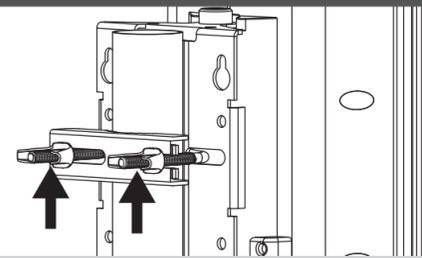
Place U-bolt through the mast, adjust the antenna bracket and fasten screws.
