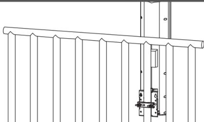
Using the U-bolt to install the antenna bracket on the railing and fasten screws.
