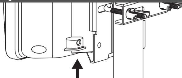
Tie a rope on the antenna hole in case the antenna falls down
