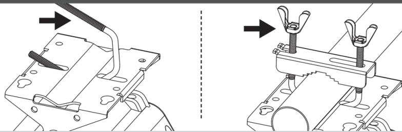
Insert the U-bolt into the hole of antenna bracket and then install the clamp in the U-bolt.
