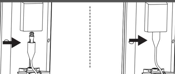
Connect the signal cable to the signal output jack of the antenna and then fix the waterproof cap covering the connections to avoid water filtration.
