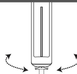
Adjust the antenna direction until you get the good signal for clear picture.
