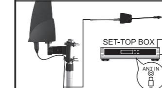
Connect the signal cable from the antenna to the signal input jack of the power supply, connect the power supply output jack to the digital receiver, plug the power adaptor with the power supply and connect to power socket, and finally join the TV and the digital receiver.
