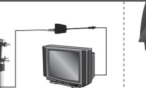
Connect the signal cable from the antenna to the digital receiver, set the receiver to offer power to the antenna and join the TV and the digital receiver.
