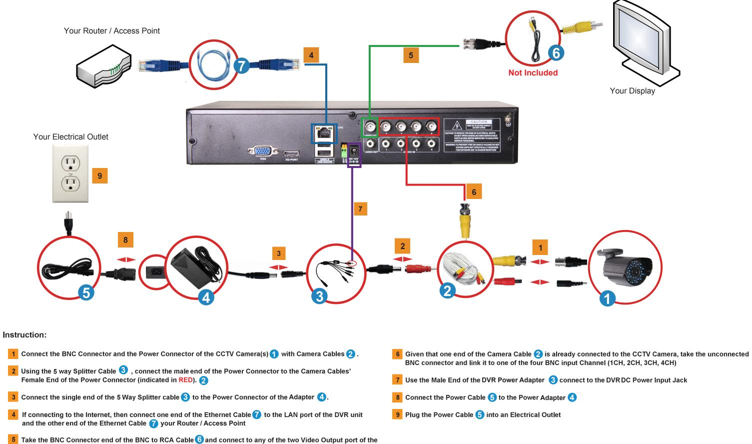
DVR unit. Take the RCA Connector end of the BNC to RCA Cable 6 and connect to the Video In RCA port of the
